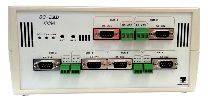
The **SC-DAD COM** is a compact smart data collection device, it can collect and treat data coming from sensors, tools, devices with output signal such as:
